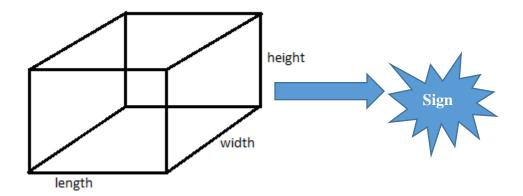
706.05-3.2 The supports, uprights or structure on which any sign is supported shall not be included in determining the sign area unless such supports, uprights or structure area are designed in such a manner as to form an integral background of the display.
